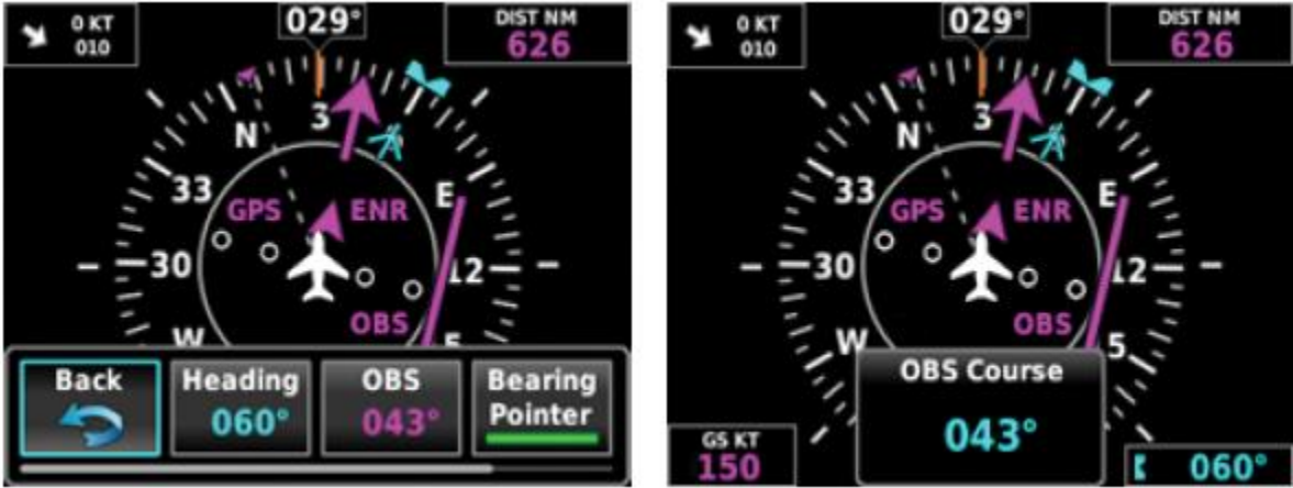
When OBS is activated on the navigator, an OBS menu option is displayed.
